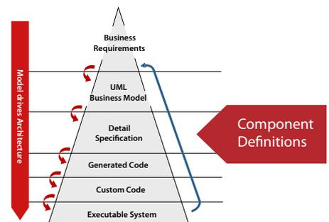
The figure above shows the MDA-based approach for Component Based Development. A key feature of MDA is the seamless transition of component models from a very high level of abstraction down to the concrete implementation.
