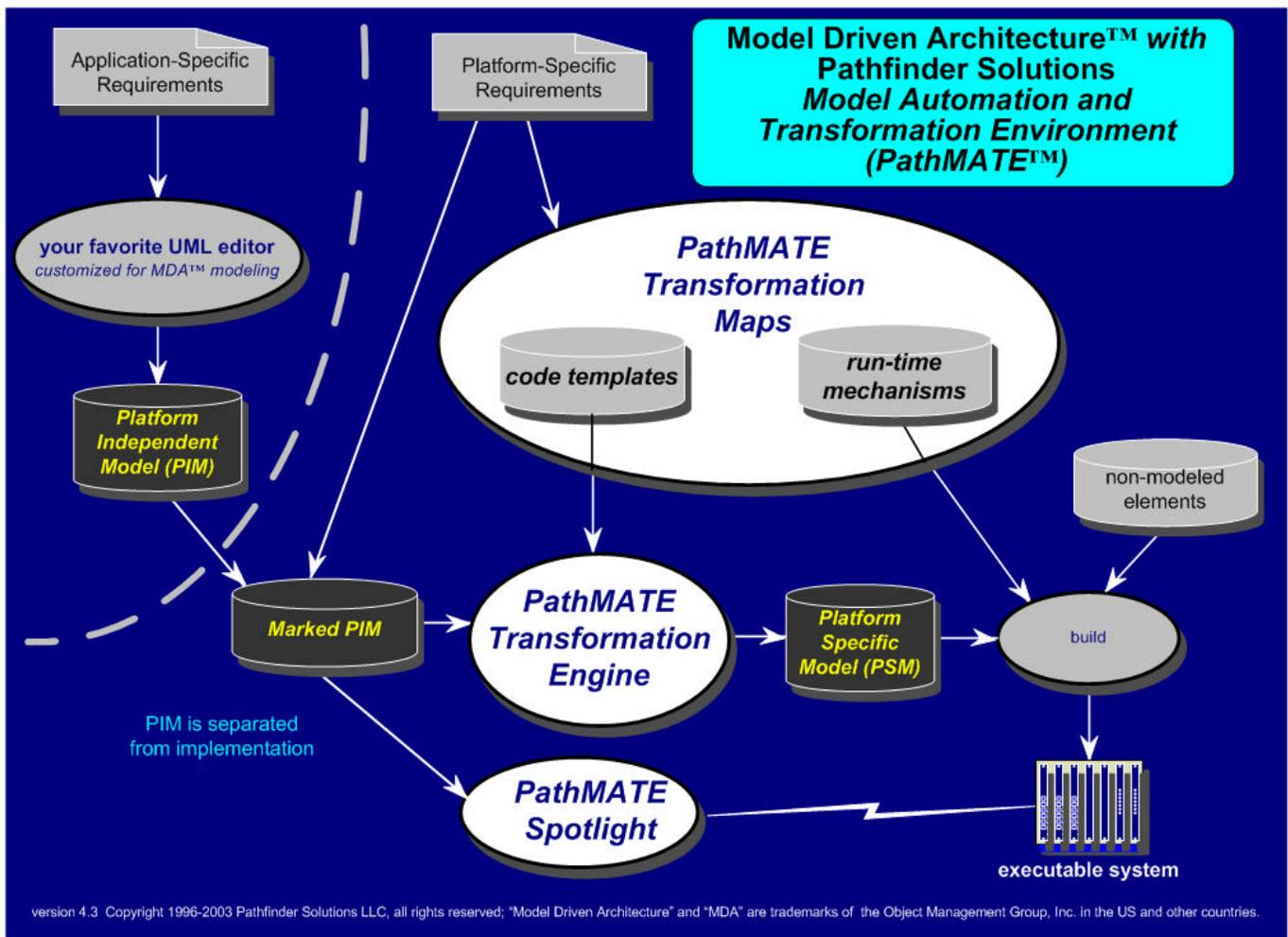
Figure 1 – MDA work flow and key technology elements
